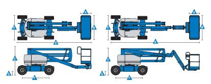
\* The metric equivalent of working height adds 2 m to platform height. U.S. adds 6 ft to platform height. \*\* In lift mode (platform raised), the machine is designed to operate on firm, level surfaces only.
